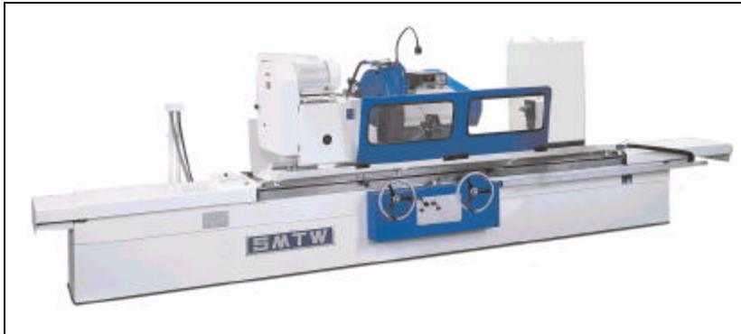
Pregrinding and postgrinding remove a total of 0.020" (0.51 mm) on diameter in a series of 0.0002" passes, all done with synthetic coolant. Pregrinding takes about six hours and finish grinding slightly longer. Both involve one belt change, from rough to finish.
