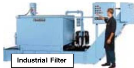
We manufacture over 60 types of filtration systems with capacities up to 560-gpm and tanks as large as 3,000 gallons. Our industrial systems remove thousands of pounds of abrasive grit and steel particles from water based coolants each day, so removing a few pounds of paint chips with copper is relatively easy stuff. Some of our other water recycling applications include: semi-truck washing, stone cutting, paint booth water-falls, potato washing, in addition to marina pressure washing.
